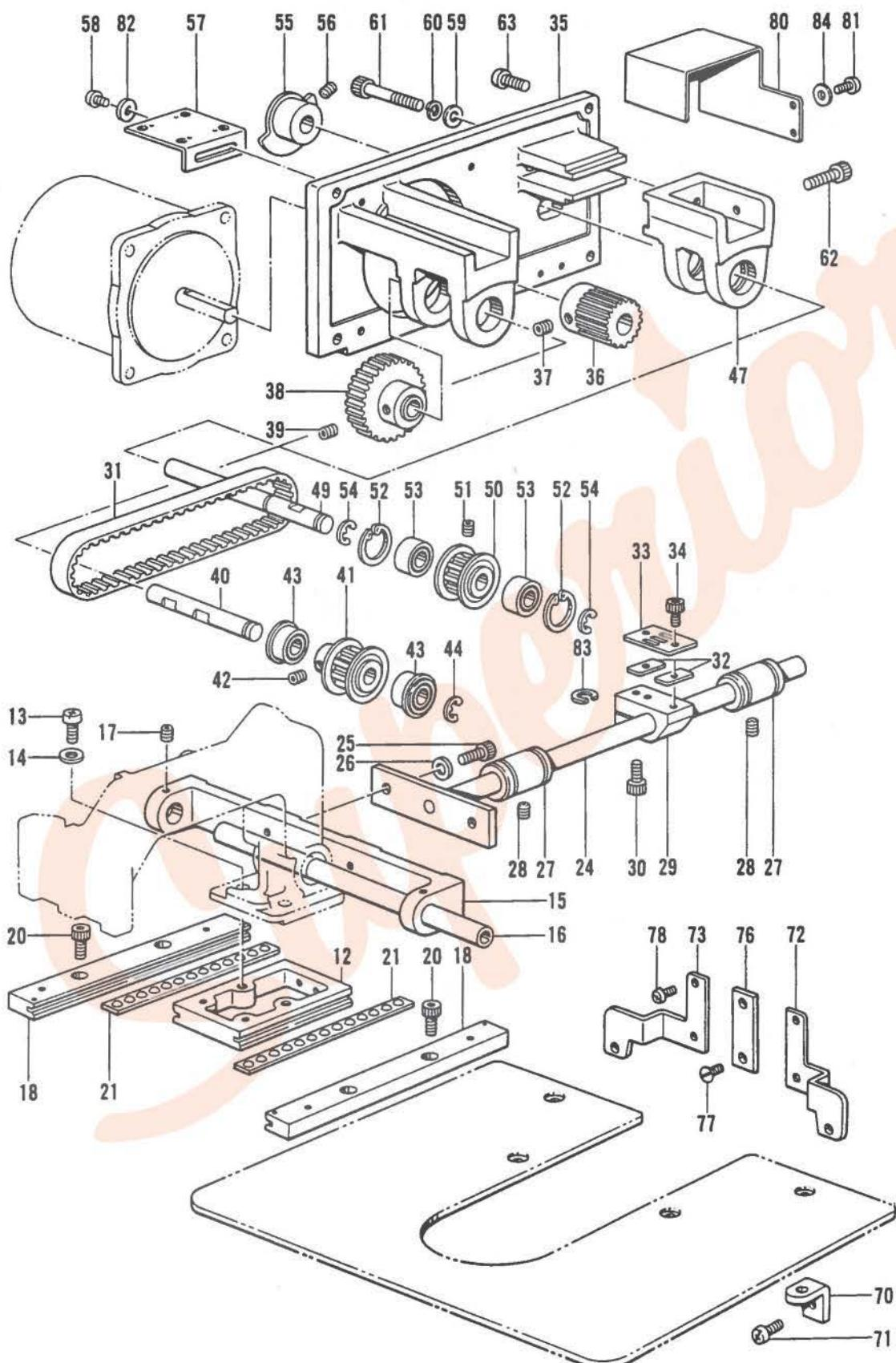
D2. 送り関係(1)/Feed mechanism (1)/Transportvorrichtung (1)/
